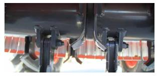
The rotor of the FXE can be equipped with universal blades or hammer blades. Lateral skids are fitted as standard.
