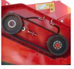
The FXZ is always equipped with a double lateral transmission. External and centralized greasing points for the rotor ensure a quicker maintenance.
