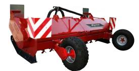
Semi pivoting wheels (10/8.0 x 12.8 ply) as standard ensure good stability and a constant working depth of the FXZ during field operations. Semi automatic linkage (Cat III) allows fast coupling of FXZ. In addition the floating top link mounting permits easy control of the working height without stressing the headstock.
