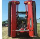
Semi pivoting wheels (10/8.0 x 12.8 ply) available as option ensure good stability and a constant working depth during field operation.
