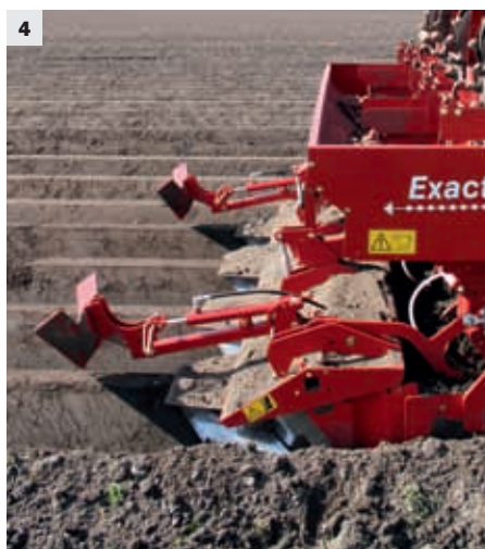
The quantity in the element (3) is very accurately controlled via sensors. After tuber placement, ridge construction is carried out immediately via the ridge shaping board (4).
