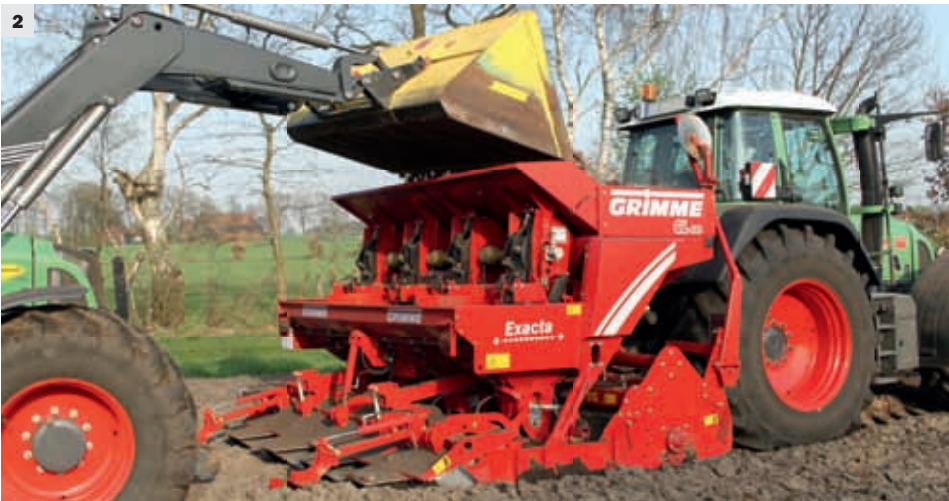
Thanks to the easy filling chute (2), it is possible to fill very gently with front loader or filling conveyor.
