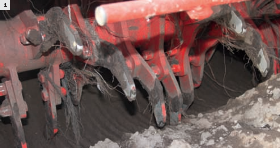
The GR 300 cultivates the full width (1). The 110 tines are arranged in spiral shape, thus guaranteeing a quiet run.
